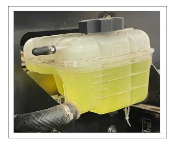
Figure 14: PROPERLY FILLED COOLANT RESERVOIR
