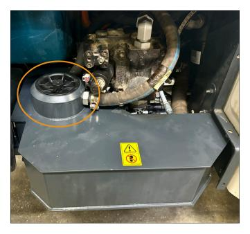
Figure 20: HYDRAULIC FLUID FILTER SHOWN INSTALLED IN THE SETTLING TANK
