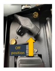
Figure 17: TURN OFF THE MAIN BATTERY SWITCH
