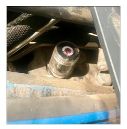
Figure 24: PRESSURE FILTER RED INDICAtor
