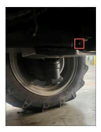
2. Use a clean cloth to wipe clean the grease fittings. It's important to keep dust out of grease fittings to avoid clogs, which can prevent grease from reaching the bearing properly.
