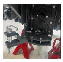
Figure 10: DRAWBAR IN LEFTMOST SWING POSITION
