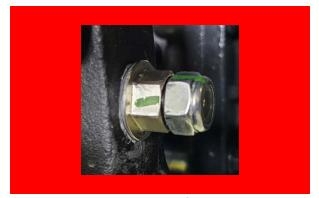
Incorrect nut placement with torque mark broken. Contact Monarch Tractor.
