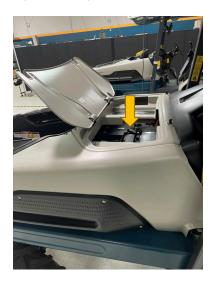
Figure 16: Accessing the Main Battery Switch
